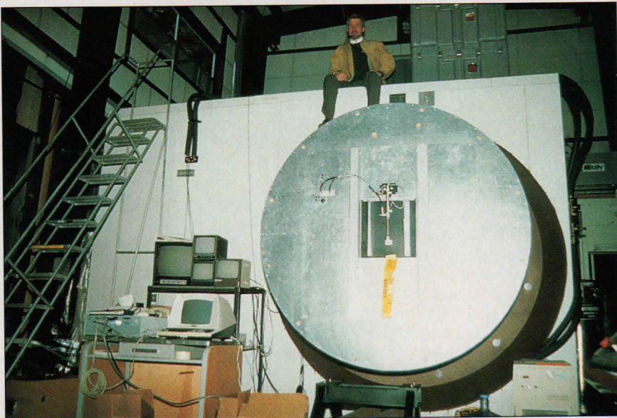
FIGURE 1. High-resolution spectrograph (HIRES) for Keck telescope is about the size of a living room. Steven Vogt, principal designer of the instrument, is seated atop the HIRES.
